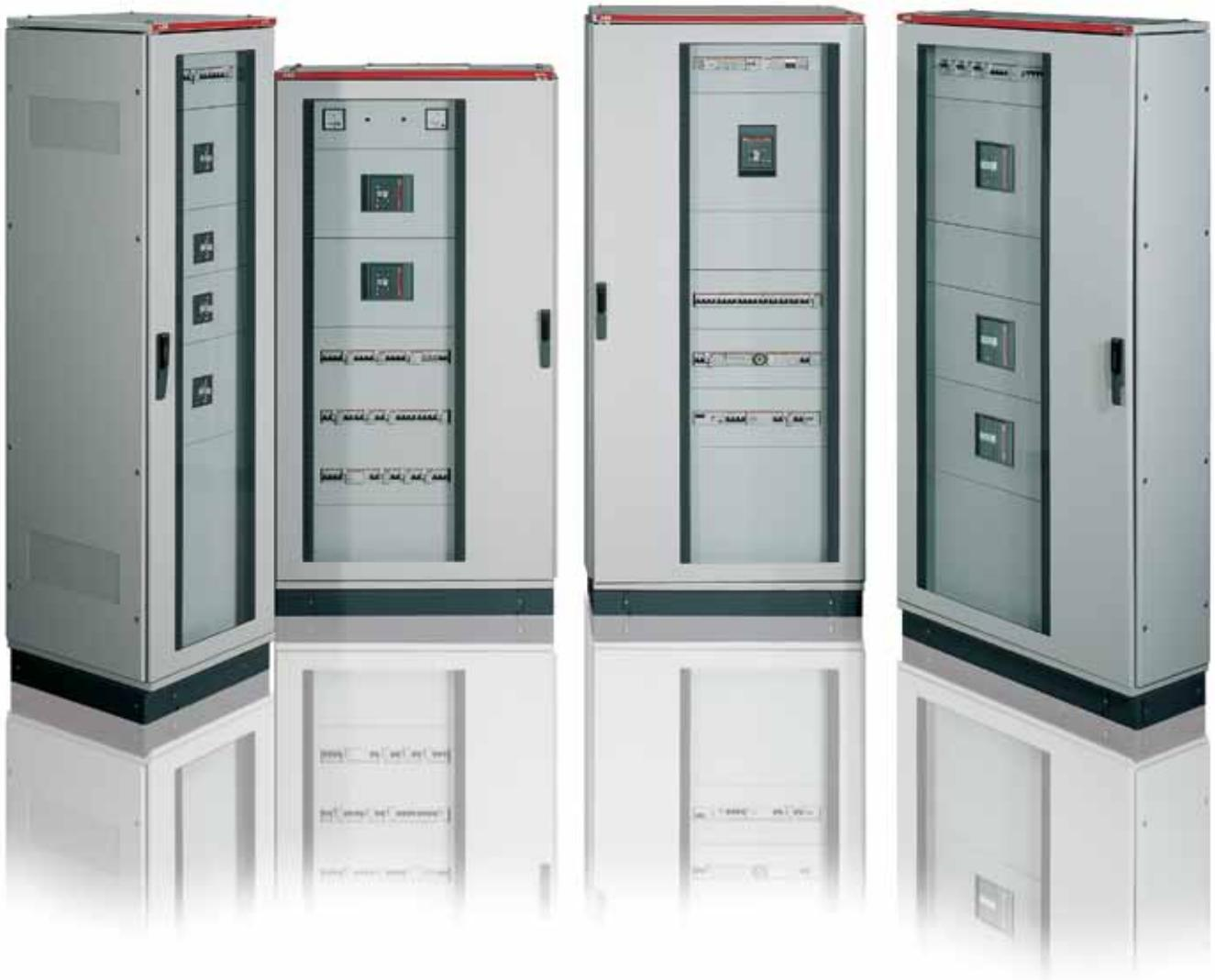
The ArTu switchgear doors are made of 15/10 steel sheet for blind versions or with 4 mm thick glass fitted with gasket able to grant IP65 degree of protection.
